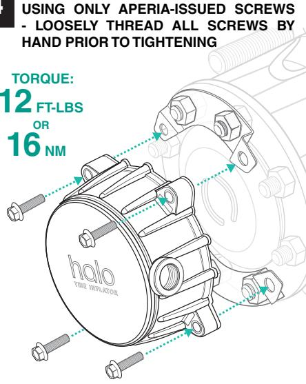
ENSURE THE HALO IS FLUSH AND WITHOUT OBSTRUCTIONS. USING A TORQUE WRENCH, TIGHTEN THE SCREWS TO 12 FT-LBS OR 16 NM.
