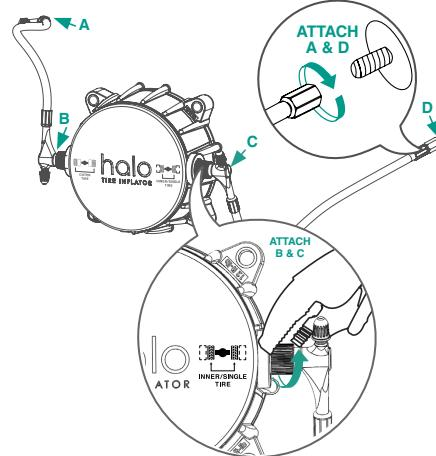
AT THE HALO, TURN THE CONNECTOR BY HAND UNTIL THE THREADS ARE SUBMERGED. USE PLIERS TO ENSURE FIT IS SNUG.
