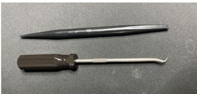
**2.** Remove the existing gasket by hooking it with the sharp pick and pulling it out the end of the hose.
