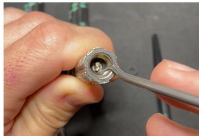
**3.** The hose end must be completely free of debris before inserting the new gasket.
