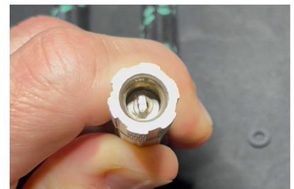
**4.** Insert the new gasket by pushing it in with the non-marring pick. Avoid nicking, scratching, or twisting the gasket.
