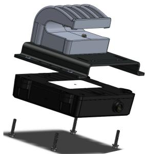
e Attach the clamp to the beam
