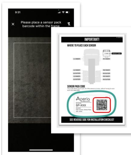
j) After the appropriate sensors have registered, select the tire position to pair a Halo
