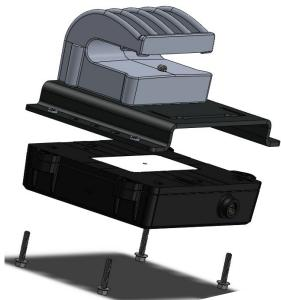
e Attach the clamp to the beam
